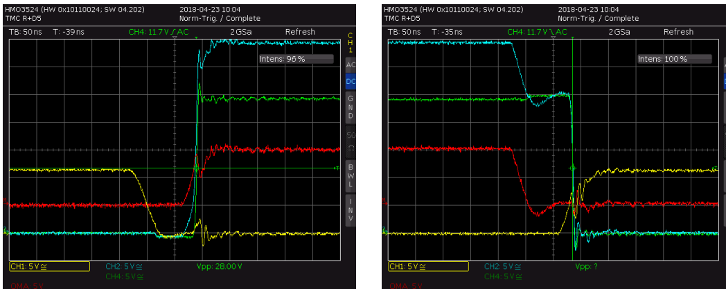
Figure 3.9 Ringing of output (green) and Gate voltages (yellow, blue) with DRVSTRENGTH=3
